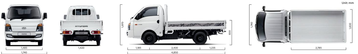
\*Above dimensions are based on standard cab extra-long wheel base pictured here
